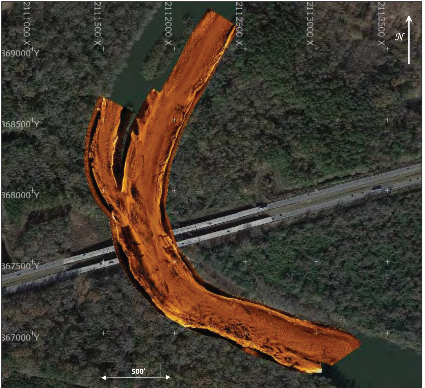
Figure 4. Sonar Mosaic of Wateree River Creek Project Area overlaid on an Aerial Photograph
