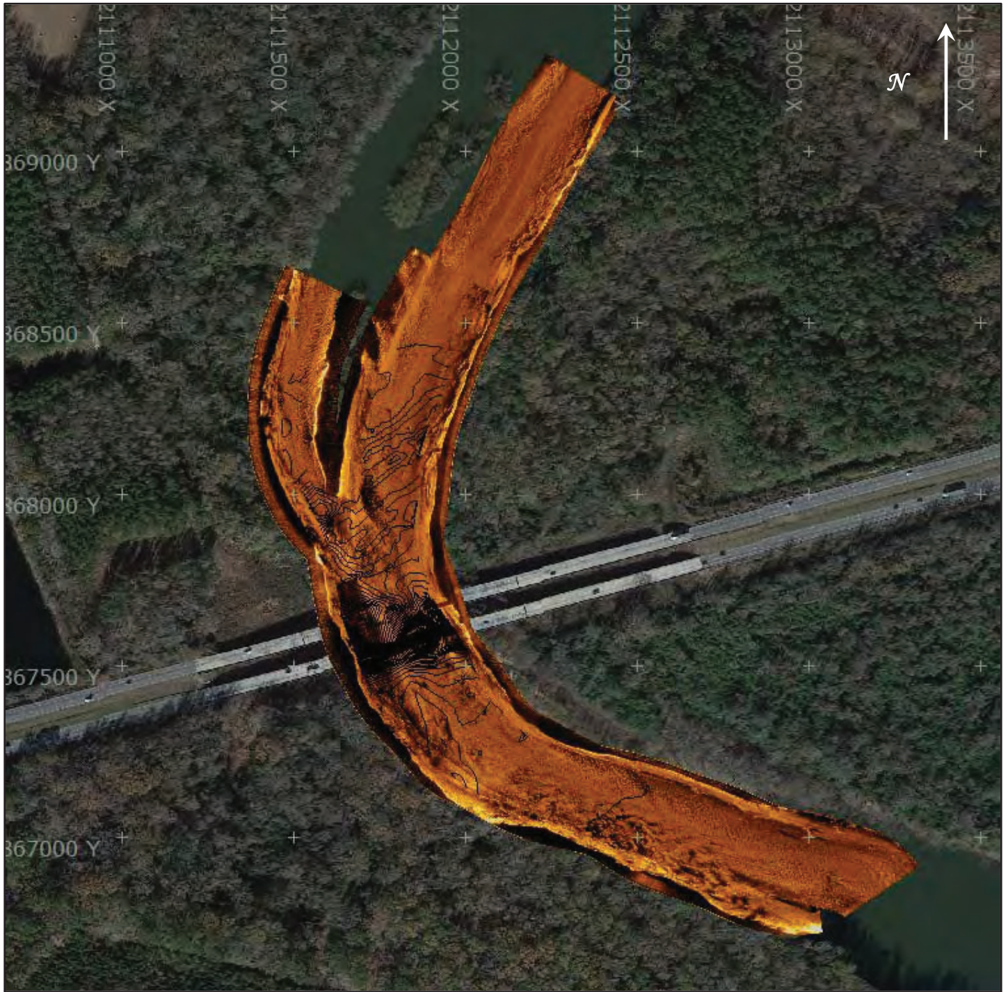
Figure 7. Sonar Mosaic overlaid with Magnetic Contours at 100 nT (gamma) Intervals
